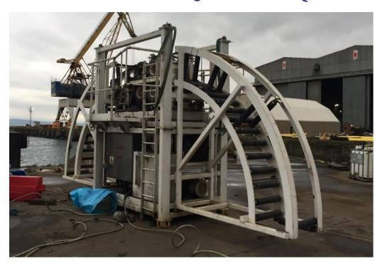
Our 2 pair powered quadrant is designed to be used in the transportation of cables both power and telecommunications. The unit is powered by an integral hydraulic power pack. The system can be concreted remotely via the control desk. The powered quadrant is an assembly of three parts; a centre frame supporting the linear cable engine (LCE), with a quarter roller quadrant bolted to each side of the centre frame.
