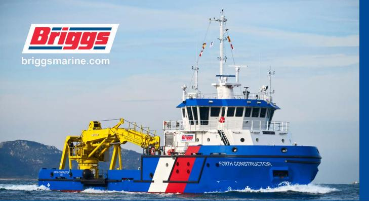
Briggs Marine's versatile Maintenance Support Vessel measures 40 metres in length and boasts DP2 propulsion as well as additional features including a heave compensated crane, a moonpool, a detachable A-frame, a 4-point mooring system, and a survey project office. Additionally, the design incorporates a demountable Crew Transfer Vessel (CTV) boarding ladder to enhance its ability to support offshore windfarm projects.
